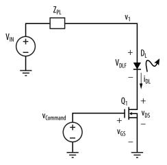
Figure 6. Simple laser driver
