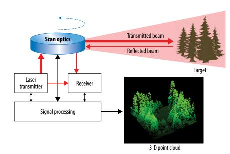
Figure 1. Basic lidar system
