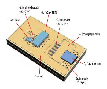
Figure 14. Typical power loop component layout.
