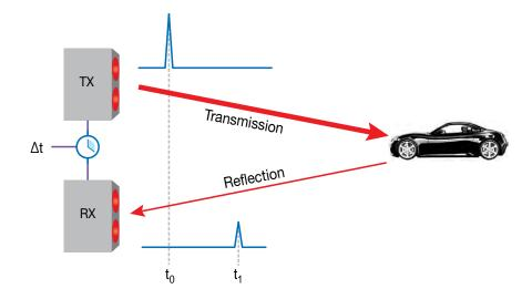
Figure 2. Simplified operation of DToF lidar system
