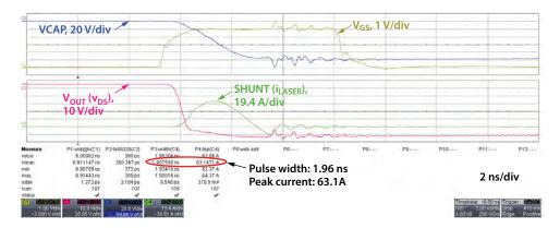
Figure 18. Waveforms for the EPC9179 demo board using an ams OSRAM SPL S1L90A\_3 A01 single channel triple junction laser diode mounted with the EPC9989 interposer.  $v_{BUS} = 70 \text{ V}$ .
