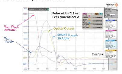
Figure 21. Waveforms for the EPC9150 demo board using an ams OSRAM SPL S4L90A\_3 A01 four channel triple laser diode mounted with the EPC9989 interposer. All channels are connected in parallel.  $V_{BUS} = 150 \text{ V}$ .
