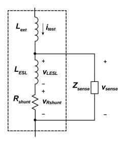
Figure 23. Current measurement shunt resistor with parasitic inductance.
