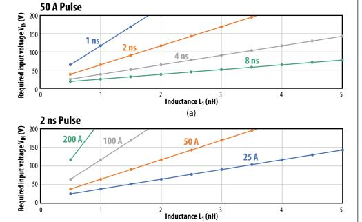
Figure 9. Bus voltage  $V_{IN}$  versus inductance  $L_{1.}$  (a) shows effect of pulse width for a specific peak pulse current of 50 A, and (b) shows the effect of current for a specific pulse width of 2 ns FWHM.
