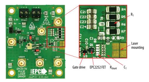
Figure 16. EPC9179 resonant pulse driver with closeup of power loop that highlights the key components of the resonant network. Inductance  $L_1$  is not shown because it is strictly due to stray inductance of the power loop components and the PCB.
