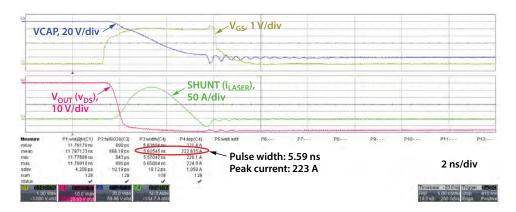
Figure 19. Waveforms for the EPC9180 demo board using an ams OSRAM SPL S4L90A\_3 A01 four channel triple laser diode mounted with the EPC9989 interposer. All channels are connected in parallel.  $v_{RUS} = 70 \text{ V}$ .
