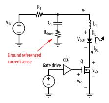
Figure 22. Circuit location of current measurement shunt in resonant pulse development boards.
