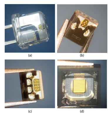
Figure 3. Some typical laser diodes used in ToF lidar systems. All diodes are from ams OSRAM: (a) SPL PL90\_3, single channel triple junction EEL, (b) SPL S1L90A\_3 A01 single channel triple junction EEL, (c) SPL S4L90A\_3 A01 quad channel triple junction EEL, and (d) EGA2000-940-W single channel triple junction VCSEL array with diffuser removed.
