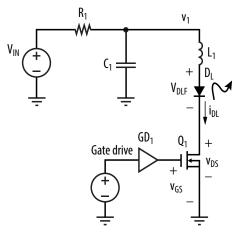
Figure 7. Simple laser driver with parasitic inductance and non-zero power supply impedance
