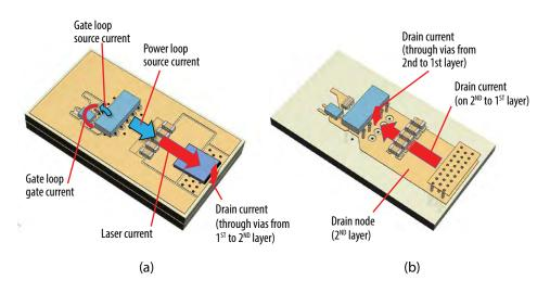
Figure 15. Physical location of power loop currents when FET is turned on
