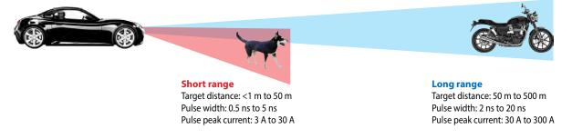
Figure 5. Typical laser driver specifications for DToF lidar systems
