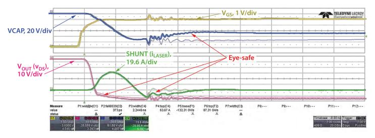
Figure 27. Comparison of conventional and fail-safe charging modes for an EPC9179 evaluation board with an ams OSRAM S1L90A 3 A01 laser installed. The thin traces show the unmodified board and the thick traces show the results with the fail-safe modification.
