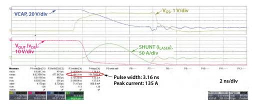
Figure 20. Waveforms for the EPC9181 demo board using an ams OSRAM SPL S4L90A\_3 A01 four channel triple laser diode mounted with the EPC9989 interposer. All channels are connected in parallel.  $v_{BUS} = 70 \text{ V}$ .
