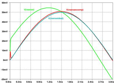
Figure 24. Simulation of current shunts and comparison of results for ideal shunt, uncompensated shunt with ESL, and compensated shunt using RC network. In this simulation,  $R_{shunt} = 100 \text{ m}\Omega$  and  $L_{shunt} = L_{ESL} = 40 \text{ pH}$ . A half-sine pulse with pulse width of 2 ns FWHM.
