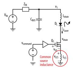
Figure 13. Laser driver showing common source inductance  $L_{CS}$
